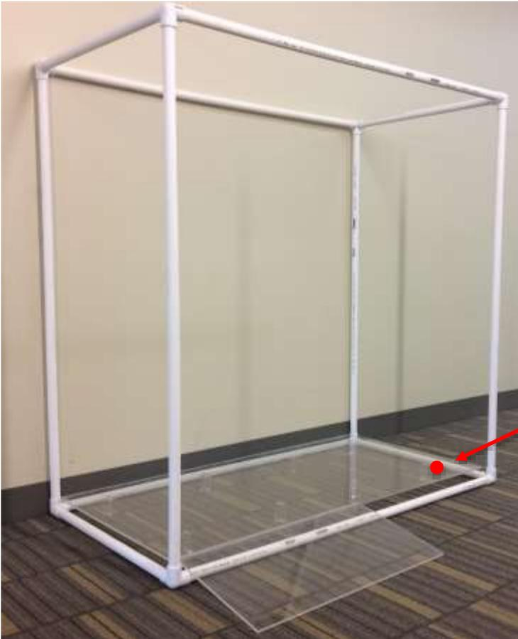
**Egg Hatchery.** During the event the walls will be covered with black fabric so that the inside is not directly visible. A camera will be mounted above and viewable on a TV monitor for navigation. The hole that eggs must be dropped in to will be in lower right corner of this image.
