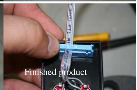
8. You can screw on the back of your remote case, making sure that the cable feeds through the slot at the top of the case. You will now move to the connector at the other end of the cable. Snap off a piece of right-angle male header containing 5 pins, and place it in your helping-hand device or into a breadboard, leaving the bent side of the pins exposed, and bent towards you. Tin each of the bent ends of the header with solder.
