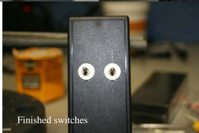
2. For the next parts, a vise or someone to hold the case will help greatly. Turn the front of the case over so that you can work with the solder lugs on the switches. Now, take one of your diodes, and hold one of the leads across the middle terminals of both switches. Cut just enough of the lead off so that it will reach across both middle terminals (if you're uncomfortable cutting your diode leads, a piece of paper clip or similar metal will also work).
