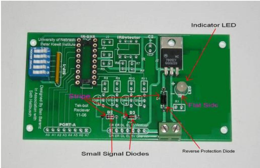
Next, place the resistors. There are six 1kΩ resistors R1, R4, R8, R9, R10, R11, two 100Ω resistors R6,R7, and one 10kΩ resistor R5. All resistors will be mounted vertically as shown in Fig 8.
