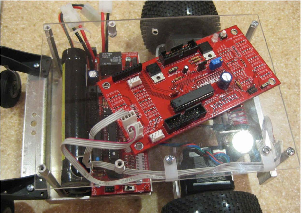
29. Attach the Interface board using three 6x32-1/4" screws except the right rear corner. Use a 1/4" M-F standoff for this corner.
