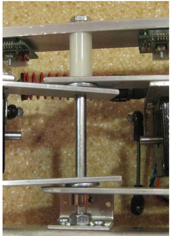
23. Working from the bottom, press the locking collar towards the front of the CEENBot to remove any excess play and tighten the set screw.
