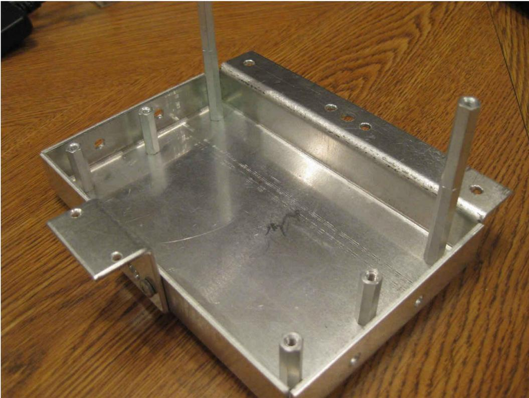
15. Disassemble all remaining parts of the tray.
