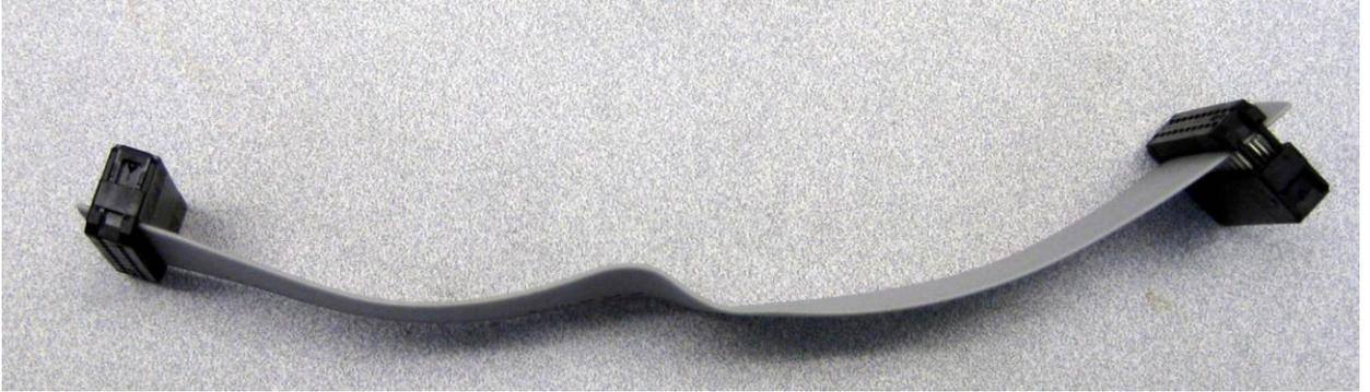
8. Connect the ribbon cable to the back two connectors on the Interface and Control boards. The plastic key will only allow you to place it one way.
