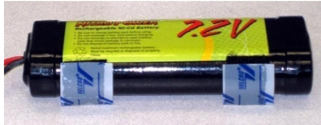
11. Carefully place the battery in its position in the CEENBoT to transfer the Velcro to the battery compartment base. Remove the battery and press the Velcro to the CEENBoT with your fingers.
