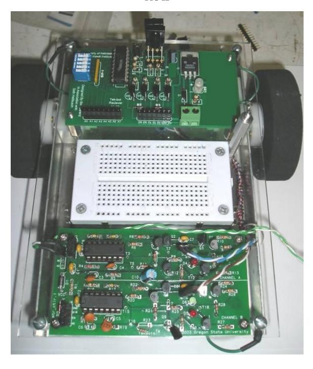
Next we will need two 2-Pin wires to connect the motor controller board to the receiver board and one 2-Pin wire for power. Cut three sets of two wires approximately 8" long. Then solder a 2-pin male header to the end of each wire as shown in Fig 13.
