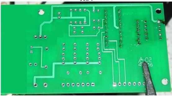
Next, place the SIP resistor with the black dot facing down on the board as shown in **Fig** 5. Then solder in the 5P DIP Switch in **Fig** 5.
