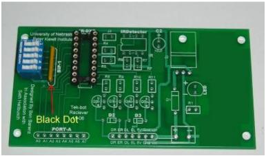
Next, place the 5V regulator and 2-Pin screw terminal. Start by bending the leads of the regulator as shown in **Fig 6a, 6b**. Place the regulator in the spot marked on the silk screen and solder. Place the screw terminal as shown in **Fig 6c** and solder.
