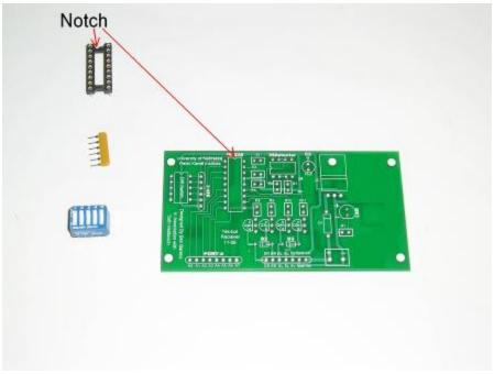
Flip the board over, then while holding the component from the back side solder the first pin in the upper corner. Apply solder then hold the iron tip on the joint for about 1 second then remove. Repeat this process for the rest of the pins as shown in **Fig 4.**
