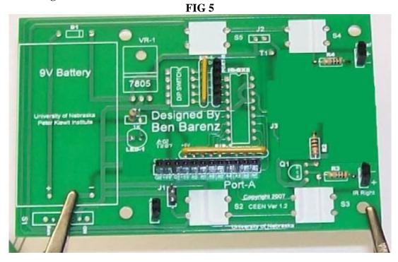
Next, place the DIP-18 Socket for the IR-DX8 followed by the DIP switch. Pay attention to the notch on the socket, and match it to the board. The numbers of the DIP switch should be closest to the SIP resistor. Continue by placing the LED-1, Q1, and the 5V regulator as in **Fig 6.** The LED has a flat spot (shorter lead is closest to it) that aligns with the board, this indicates polarity.
