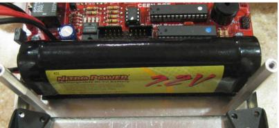
28. Attach the Plexiglas to the six standoffs. Use 6x32-1/4" screws on the front and  $\frac{1}{4}$ " standoffs on the back four.
