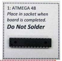
Dashed outlines mean component orientation is critical \*The single slot in the housing aligns with silk screen marking
