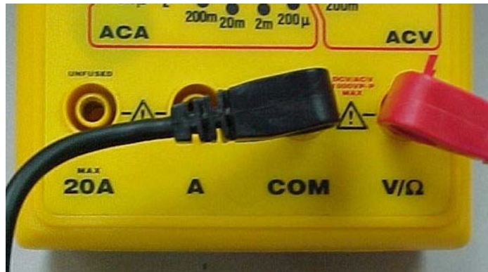
Figure 3. The positioning of the probes on a DMM for measurement.
