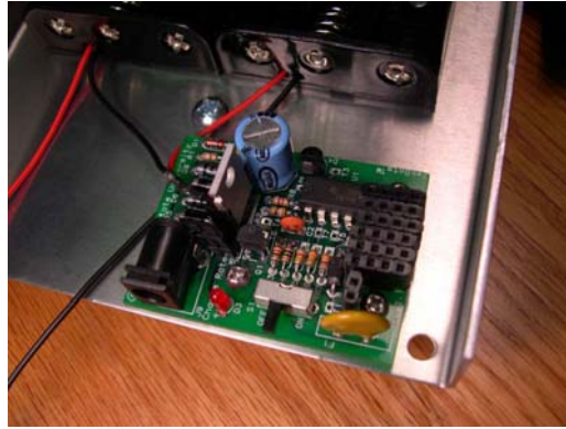
Figure 5: Diagram of spacer usage and base with connected charger board.
