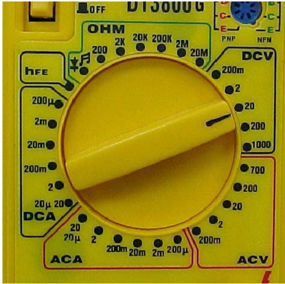
Figure 2: The settings dial on a common DMM.
