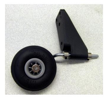
Mount the tail wheels to the tail ledge with 6x32x1/2" bolts and nylon lock nuts. They can be mounted pointing back or to 45° to the side. For now, mount pointing to the side because the CEENBoT will fit into its box.
