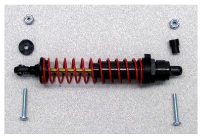
Mount using 6x32x3/4" bolts and nylon lock nuts. Note the placement of the black plastic washer.
