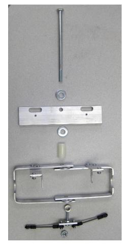
Assemble kingpin parts. Tighten nut so that it is snug but the sway bars still can move freely.
