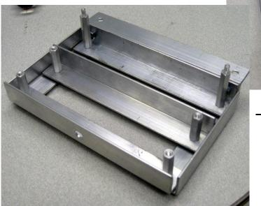
Mount the shock towers to the sway bars as shown. The view is from the front of the CEENBot. The half-moon cutouts are to the top. The left shock tower is mounted by screwing two 6x32x1/4" bolts
