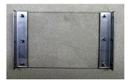
Place the angle aluminum as shown. The piece with the center hole is on one end (the front) and the double piece is on the other. Note the location of the screws on the rear piece. Secure by screwing four 7/8" female-female standoffs onto the 6x32x1/2" bolts on the front section and with two 1 ½" female-male standoffs on the rear.
