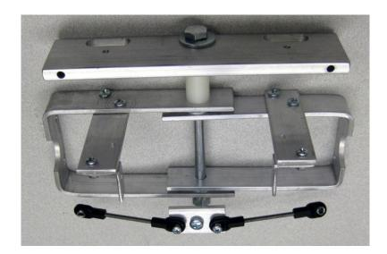
Attach the stabilizers to the shock towers using 4x40x1/2" bolts and locking nylon nuts. You will need to adjust the lengths of the stabilizers so that the mounting plate is parallel to the sway bars. Tighten the 1" bolt in the lock collar.
