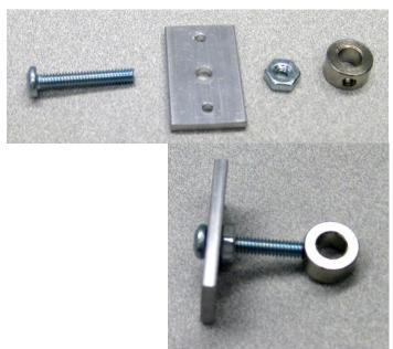
Mount the sway bars to the shock mounting plate with 4x40x1/2" screws and 4x40 nylon locking nuts.
