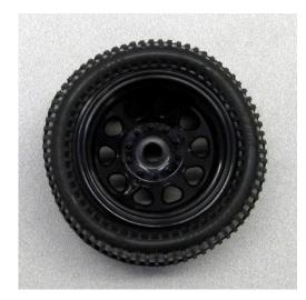
Work the tire over the wheel and adjust so that the tire bead is adjacent to the outer flange of the wheel.
