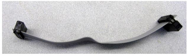
Connect the ribbon cable to the back two connectors on the Interface and Control boards. The plastic key will only allow you to place it one way.
