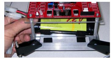
12. Place the 15" cable from the left sensor board to connector S1 on the Interface board. Place the 11" cable from the right sensor board to connector S0 on the Interface board. Route the wires through the cable holders and the hole in the rear of the Plexiglas.
