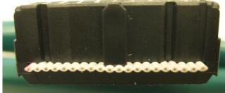
7. Attach the second connector to the other end. The plastic key goes to the stub end. The female sockets of one connector will point up and the other will point down.
