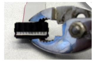
When completed, the plastic of the top part should be against the plastic of the other part.
