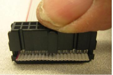
even pressure on the surface. Needle nose pliers usually do not work well.
