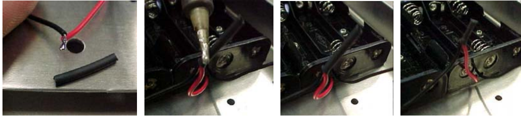
Figure 5: The step for shrink tubing a connection.
