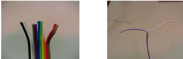
Figure 1: Ribbon cable used to connect motors.
