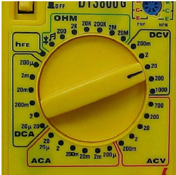
Figure 2: The settings dial on a common DMM.
