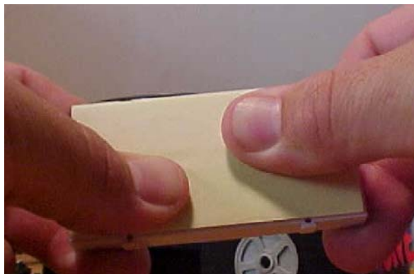
Figure 5 Seating a Breadboard's Contacts
